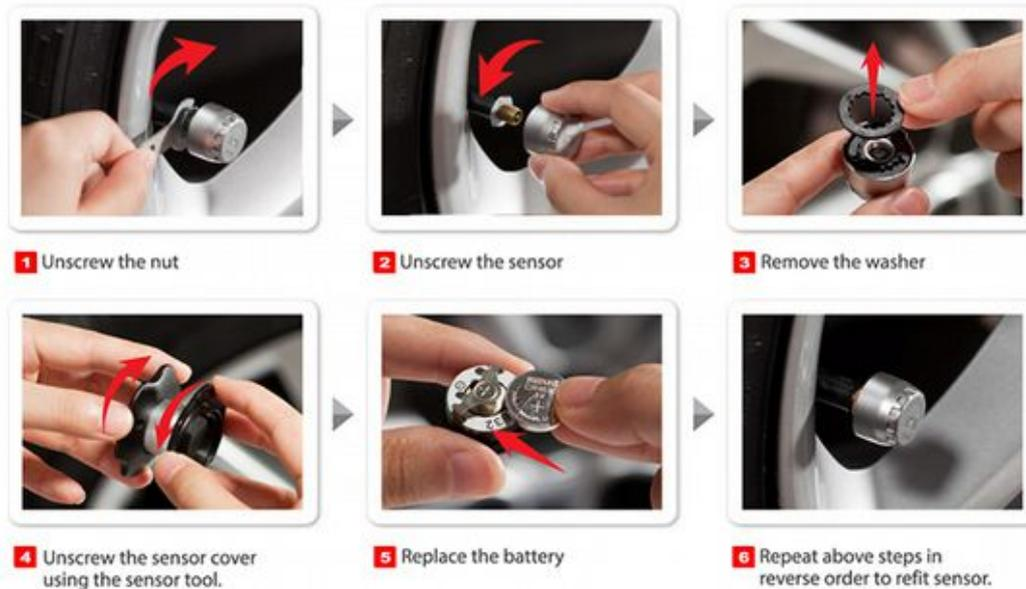
**Note:** The above picture is just for reference, in the 4th photo, we don't need the 'sensor tool' in the photo, just unscrew the sensor cover with your hands and nut wrench in the package easily.
