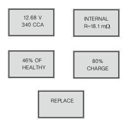
The battery is near to or already reached the end of the using life, replace battery, otherwise, bigger danger will be followed.
