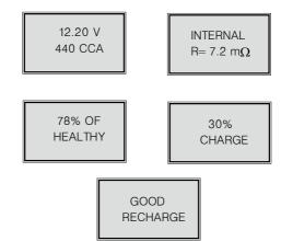
Good battery but low current, recharge before using. (Healthy>60%, Voltage>12.4V)
